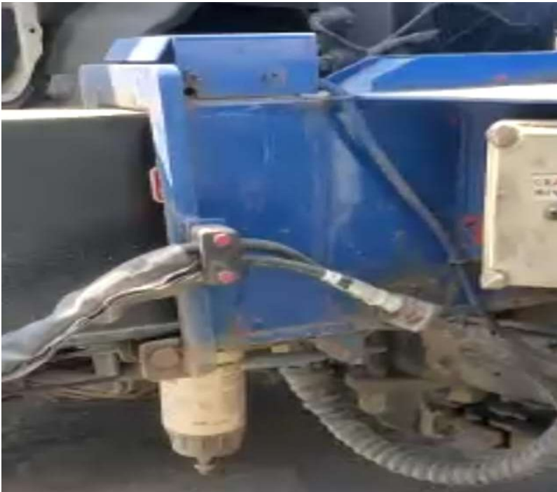
Pic-2 Bolting of chassis of vehicle and beam of boomlift just behind the vehicle cabin from upper right side
