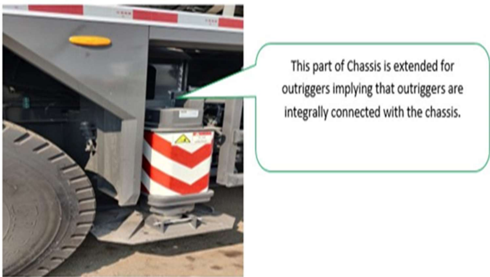
Pic-6 This picture shows the front side right outrigger of the crane.
