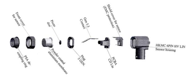
**2.13** It could be seen that an ultrasonic sensor is essentially a semiconductor (piezoelectric) -based transducer that converts a physical phenomenon into a corresponding electrical signal and vice-versa.
